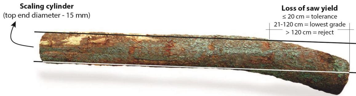
Figure 1. Determining loss of saw yield.
